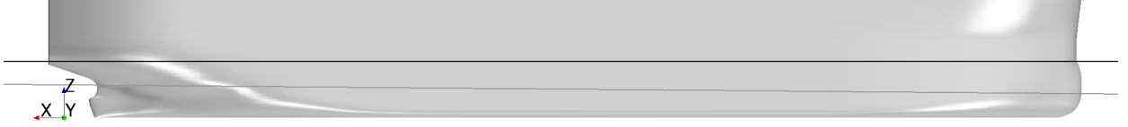
Figure 3.2: Hull geometry. The black line is the water line of the design condition, and the grey line is the water line of the sea trial condition. Seen from starboard side.
