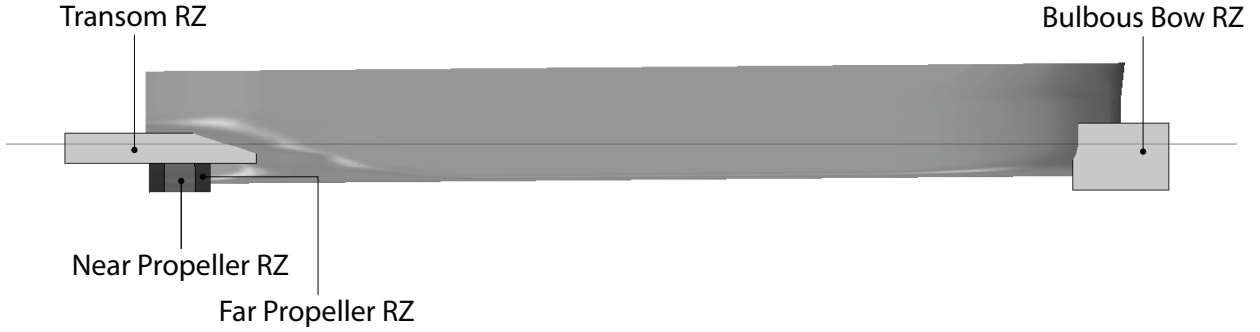
Figure 3.35: The four refinement zones of the self-propulsion setup. Seen from starboard side.
