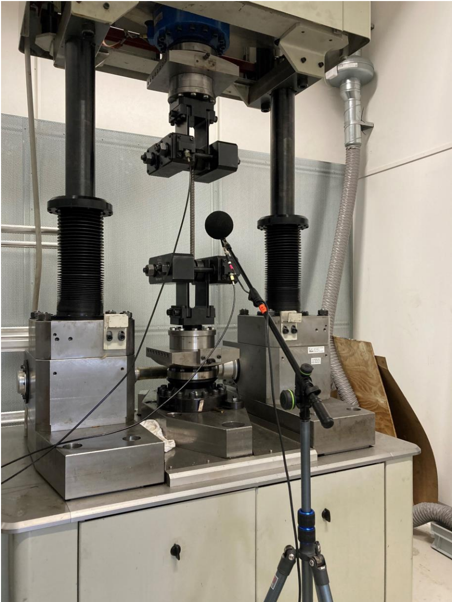
Figure 1. Principle of the acoustic emission wave detection.
