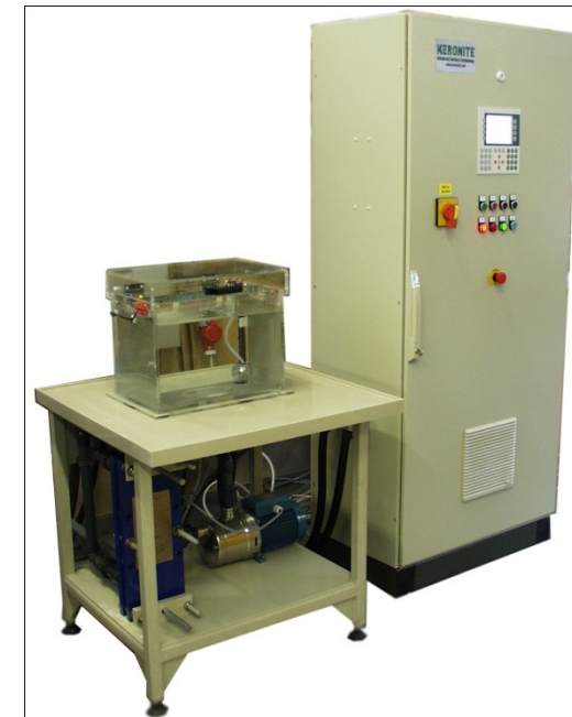
Research & Development Unit (10 kW, 25 litres bath)
